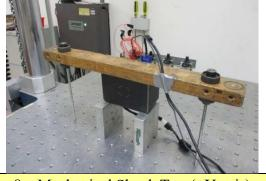
Mechanical Shock Test (-X axis)
